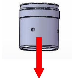
Pay attention to the direction when assembling the disc spring, as shown in the figure below:
